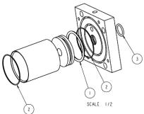
Figure 44: PR70 Air Cylinder Rebuild Kits, 4.5" and 3.0" Diameter Versions (LC0092 & LC0091).
